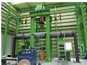
Testing device for bending pile
