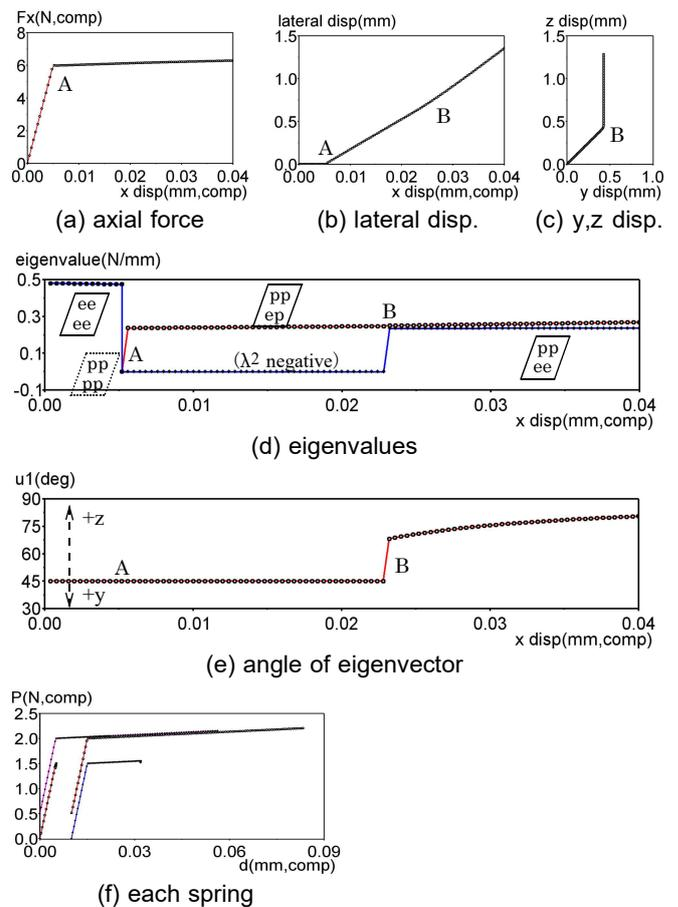
Fig. 2 Results of spring column model
