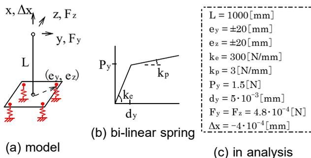
Fig. 1 Spring column model
