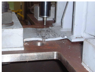
Photo.3 Buckling of a wing
